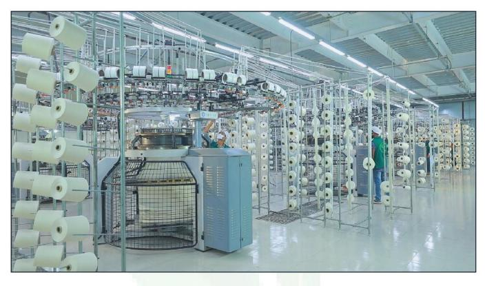
Its state-of-the-art Knit Circular machines, produce knit fabrics for its own consumption.
